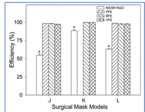
Bacterial filtration efficiency (BFE) and viral filtration efficiency (VFE) are other filtration measures that evaluate larger aerosols under less severe test conditions. As such, although they may be optionally presented by the manufacturer to supplement the required NIOSH-based tests, they too will generate results that are much higher, but not comparable.
